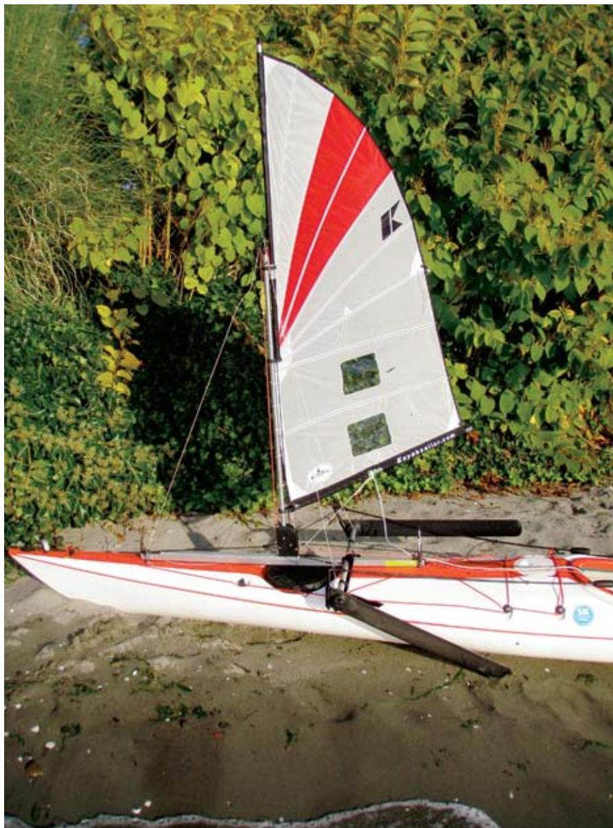
Kayaksailor 1.4 on a Tahe Wind 505, a kayak with a beam a shade over 21 inches. The sail manufacturer recommends a wider kayak for greater stability, but I thought I'd poke the edge of the envelope with a narrow boat. Once I had the rig mounted, I left it on the kayak, loaded it all up on the roof rack and headed to the water.
