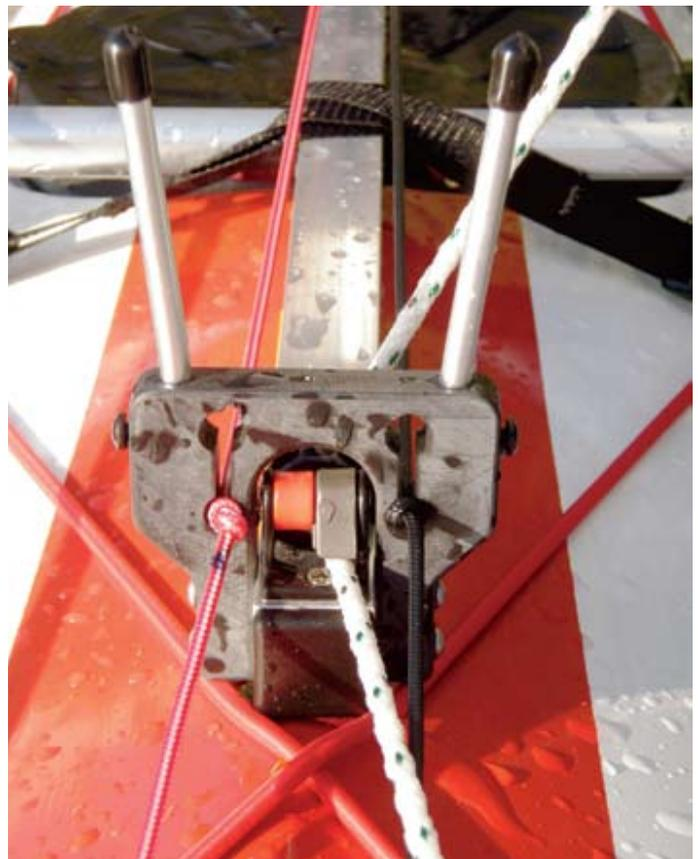
after leaving the beach the rig tilted to one side. I paddled to a dock, got out of the kayak and readjusted the crossbeam straps. I hitched the tail ends around the webbing between the padeye and crossbeam and that helped lock the cross beam solidly in position.
